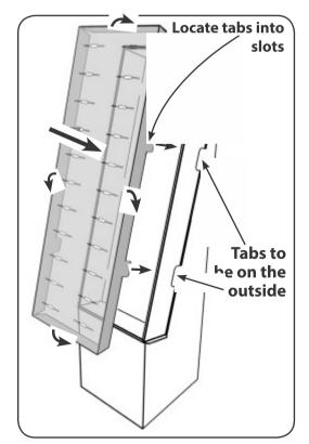
Fold end flaps of the pegboard then insert into the cassette.
