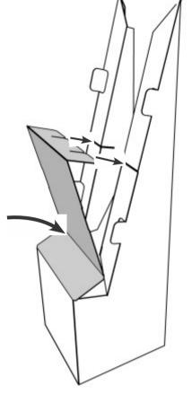
Fold over the front flap ensuring the top tab locates into the slots on the core side flaps as shown.
