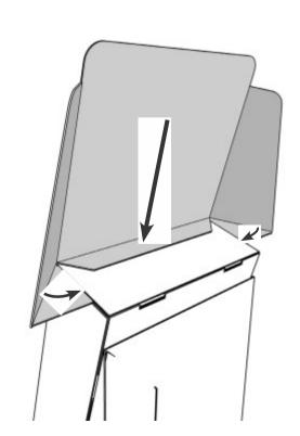
Attach the header to the unit by inserting the header onto the top slots of the cassette.
