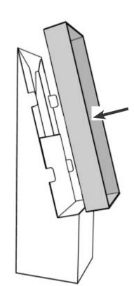
Attach the cassette to the core by allowing the tabs on the core to pass through the slots on the sides of the cassette.
